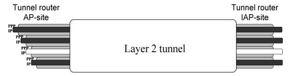
Figure 6: Layer 2 tunnel shared by multiple users
