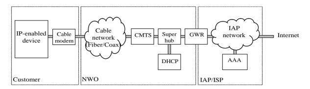
Figure 4: Cable modem access
