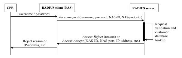
Figure A.3: Basic authentication message exchange
