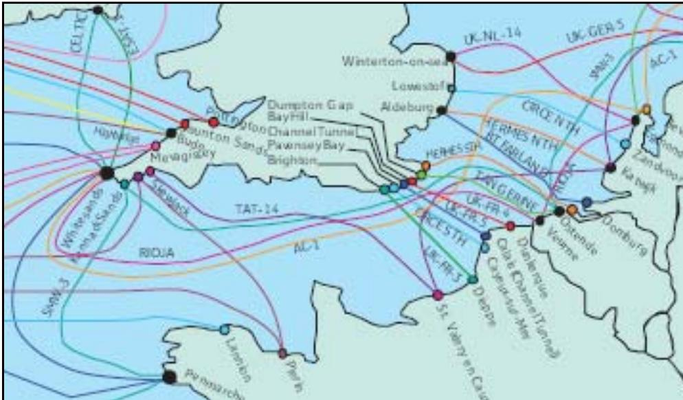
Figure 6 Map of repeaterless cross-Channel cables
